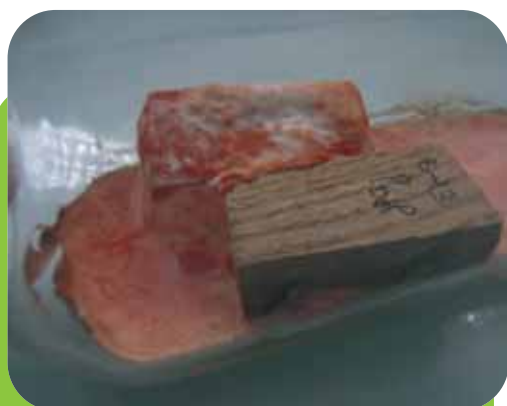
Test of the natural resistance of mulberry wood to the tropical fungus Pycnoporus sanguineus . © N. Leménager, CIRAD
