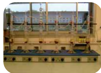
Extracting secondary metabolites from wood using Soxhlet apparatus. © N. Nkolo, CIRAD
