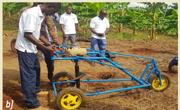
Figure 1. Examples of equipment prototypes developed for hole digging (making holes prior to planting) for plantain
