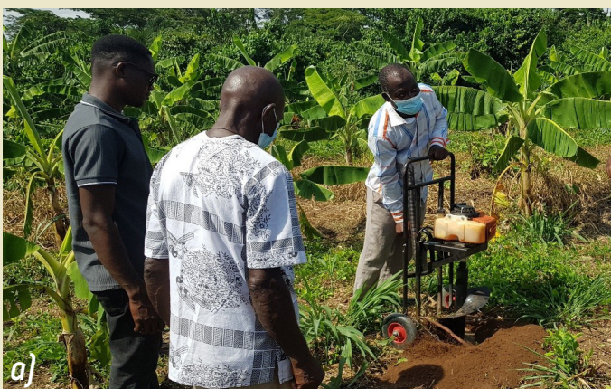
Figure 1. Examples of equipment prototypes developed for hole digging (making holes prior to planting) for plantain
