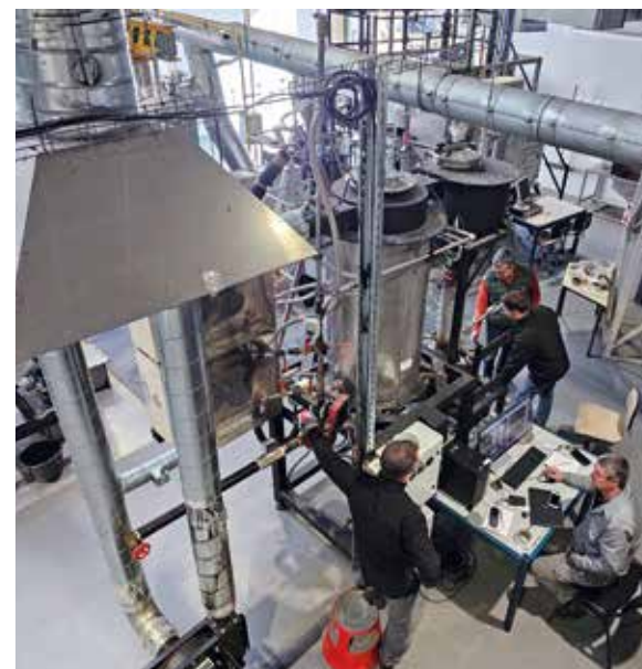
Design and development of an energy production reactor using agrifood waste, in the Biomass Energy Facility (CIRAD Montpellier) © D. Josserond, CIRAD
