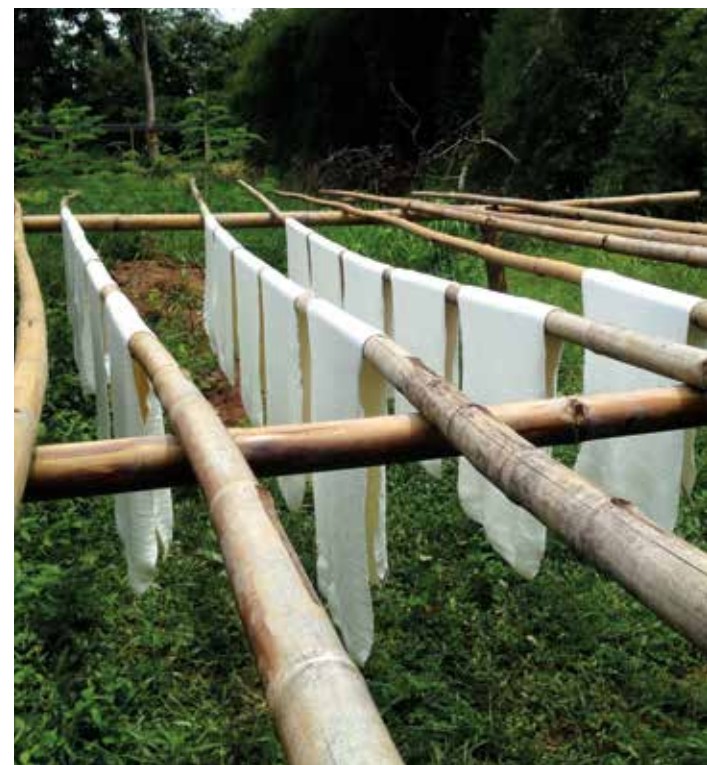
Following latex dilution and controlled coagulation by adding formic acid, the cup lumps are rolled. The resulting natural rubber sheets are hung over bamboo poles to dry in the open air. Kasetsart University Research Station, Thailand © C. Bottier, CIRAD
