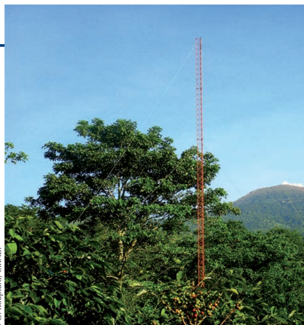
Measuring CO 2 flux above a coffee-based agroforestry planting, Costa Rica.
