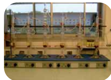
Extracting secondary metabolites from wood using Soxhlet apparatus. © N. Nkolo, CIRAD
