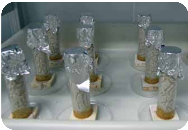
Termite resistance trial. © N. Leménager, CIRAD
